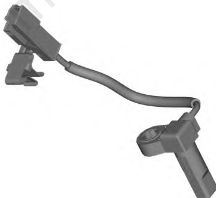
Fig. 10: Automatic Transmission Output Speed Sensor Courtesy of GENERAL MOTORS COMPANY
